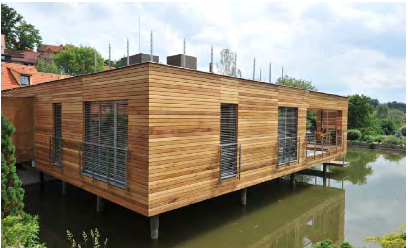
REAL FACADE Dark Red Meranti, RAUTE profile 20 x 90 mm, surface treatment OSMO UV Protective oil transparent n. 420
