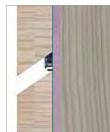
The size of the dilatation gap will be automatically set by the head of the screw.
