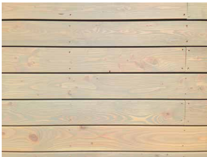
Detail of REAL FACADE, Silesian larch, Raute profile 18 x 110 mm, surface treatment OSMO single coat stain HS plus n. 9212 Silver poplar
