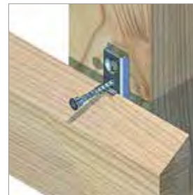
Fasten the profile to the beam.
